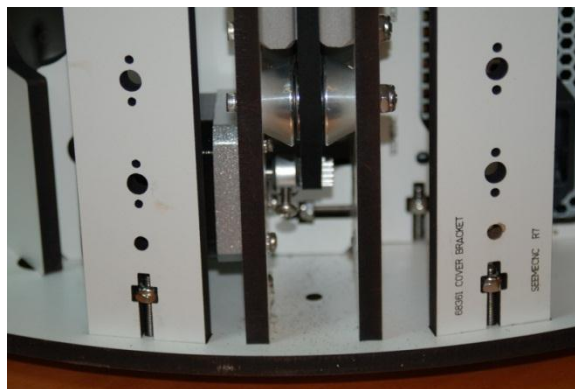
Figure 83 - Properly Aligned Pulley with Belt Installed.
