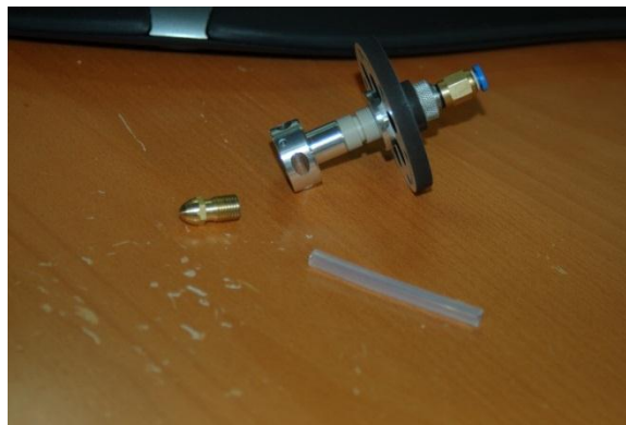
Figure 102 – The Teflon Liner ready for installation.
