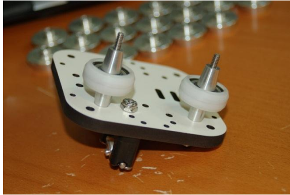
Figure 62 - Last Spacers Installed
