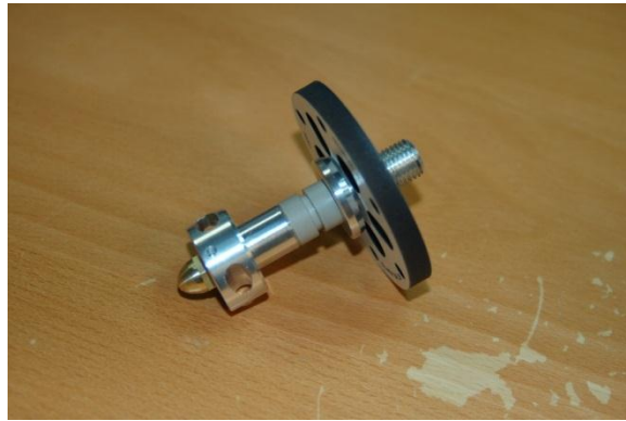
Figure 99 - Hot End Adapter Plate in position.
