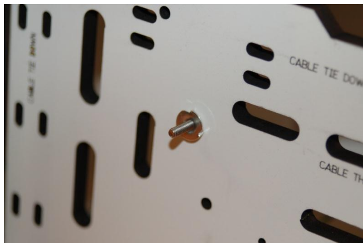
Figure 25 - Installing the T-nuts, back side
