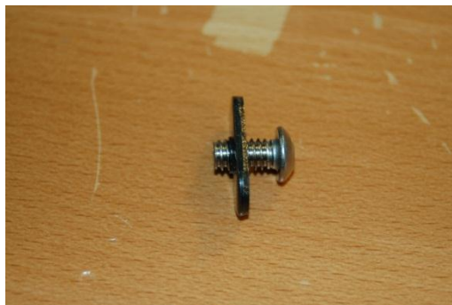
Figure 28 - Orientation of T-Nut Boss
