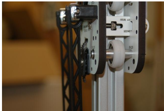
Figure 81 - Belt Clamp Installed
