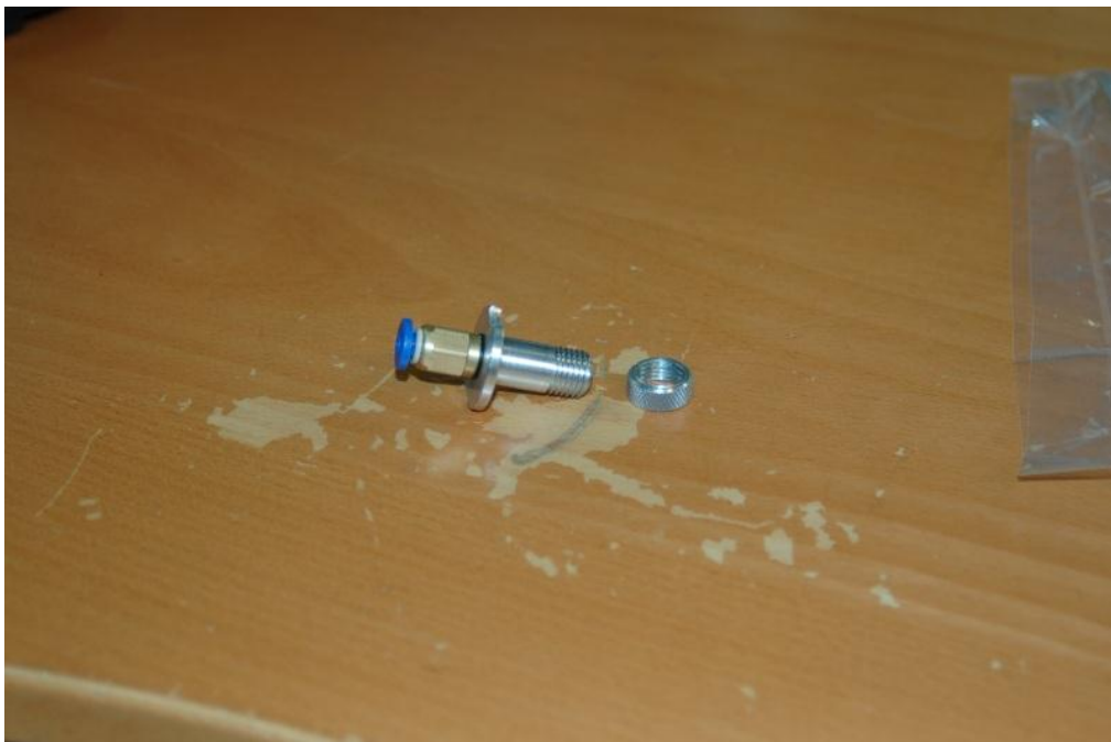
Figure 44 - Bowden fitting on Bowden Drive PTC Adapter
