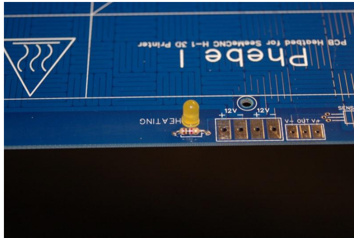
Figure 94 - Power LED installed.
