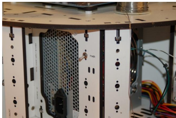
Figure 115 - Power switch installed.
