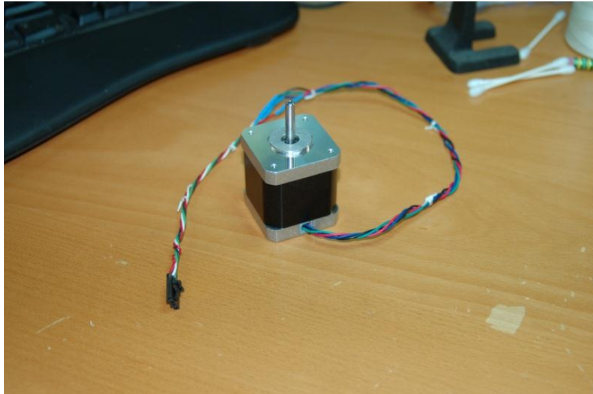
Figure 21 - Stepper motor with connector installed
