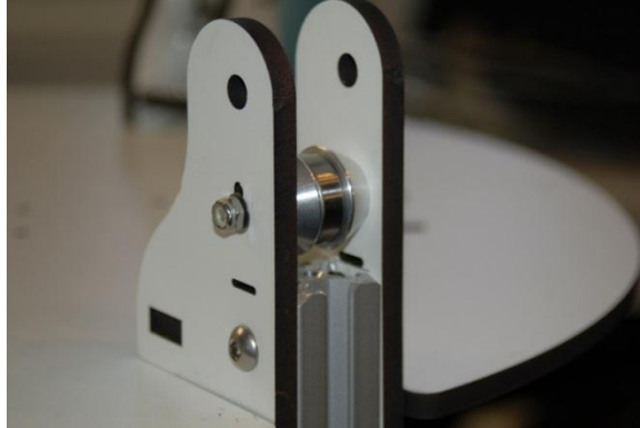
Figure 78 - Upper Idler Bearing Installed
