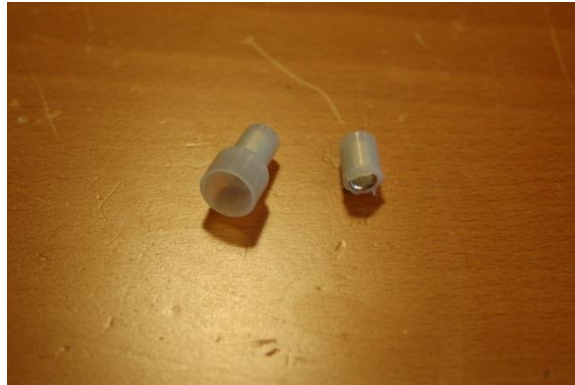
Figure 108 - Skirt trimmed from the crimp-on wire nut.
