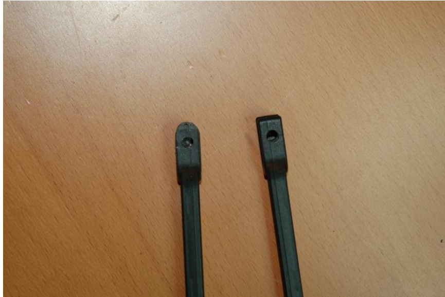
Figure 51 - Radius Sanded in Arm End.
