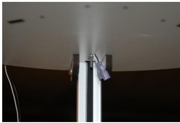
Figure 87 - Top End Stop wiring shown from the bottom.
