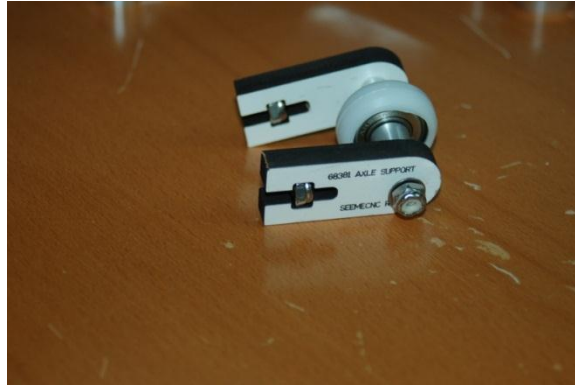
Figure 71 - Axle Support with Lock Nuts Installed
