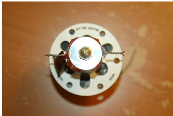
Figure 106 - Resistor wires wrapped together.
