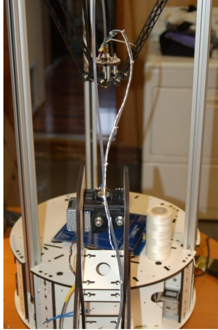
Figure 121 - Hot End heater and thermistor wires tied together.
