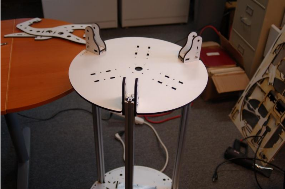
Figure 36 - Top Support Plate Installed
