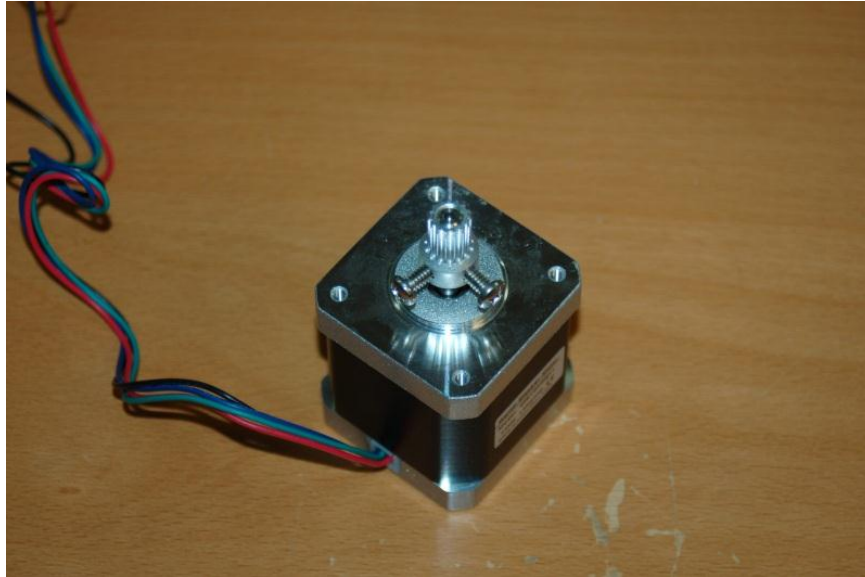
Figure 19 - Belt Pulley Installed
