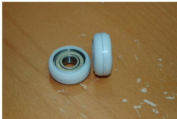
Figure 59 - Bearings with Acetal Sleeve Installed.
