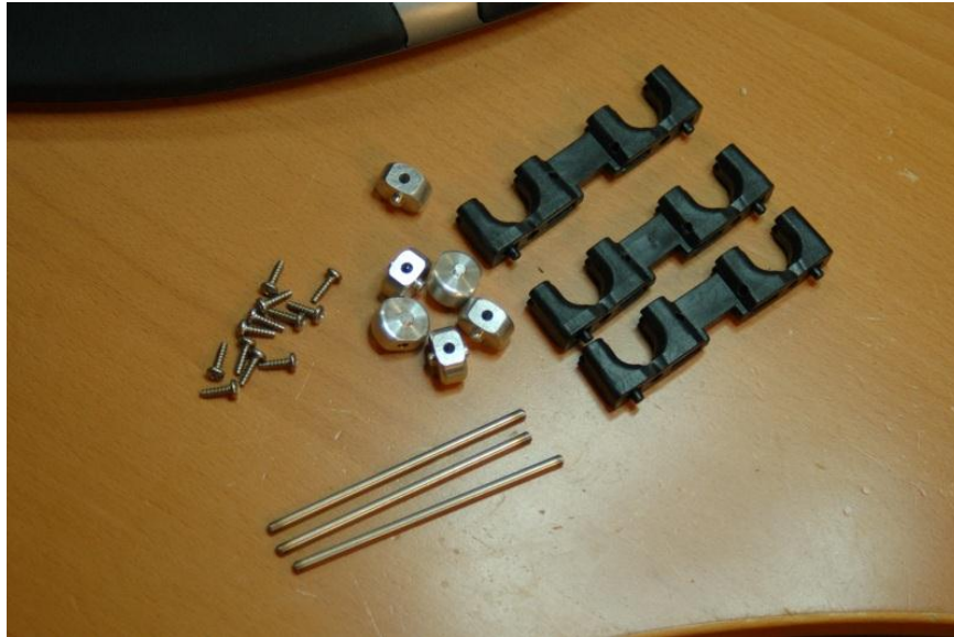
Figure 53 - Carriage U-Joint Mount Parts.
