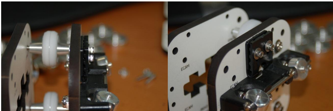
Figure 67A & Figure 67B – Upper Belt Clamp Installed
