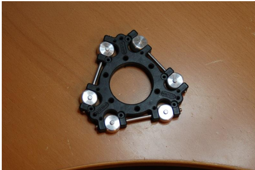
Figure 48 - U-Joints and U-Joint Axles Installed.
