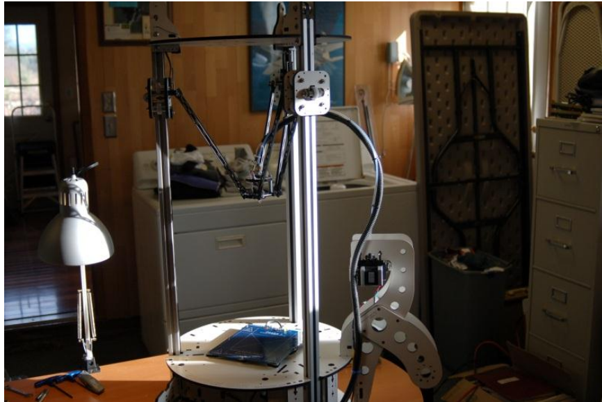
Figure 123 - Split Flex Tubing installed on Hot End wiring.
