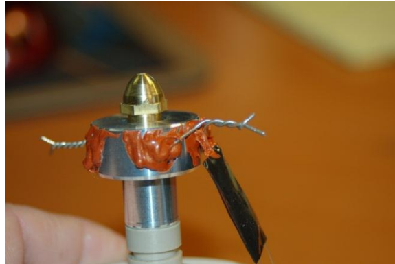
Figure 105 - Resistor wires wrapped together.
