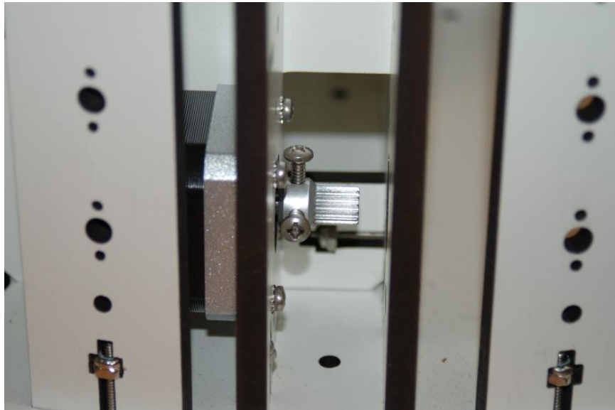
Figure 22 - Pulley correctly installed
