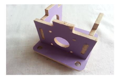
Apply PVA glue to the contact areas and glue onto the ply wood build platform. Align the ply wood so the side with the nicest finish is away from the motor mount.
