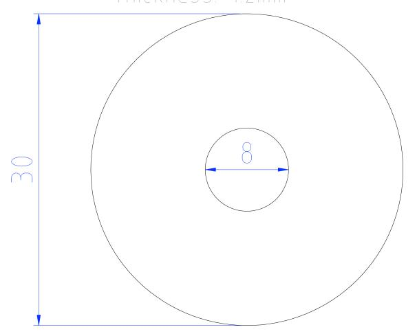
End plate (2x) thickness: 1.2mm
