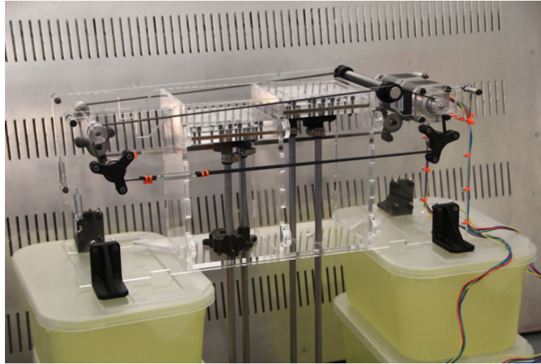
Figure 9. The prototype hardware during assembly.
