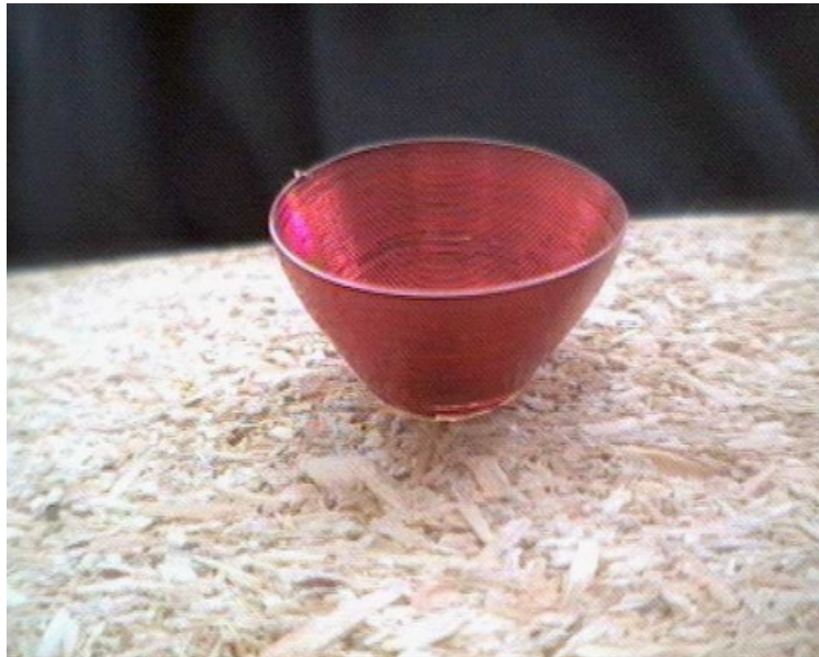
Figure 5: A part printed entirely from wire. (Image courtesy of Dany Lipsker, Micromod Technologies).
