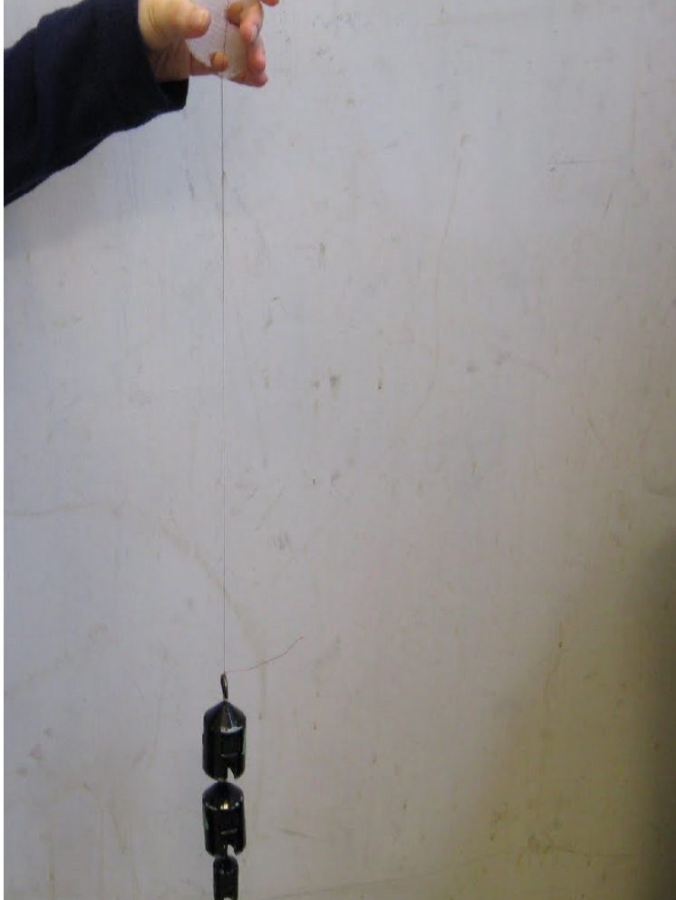
Figure 16: Test of wire-plastic bond strength
