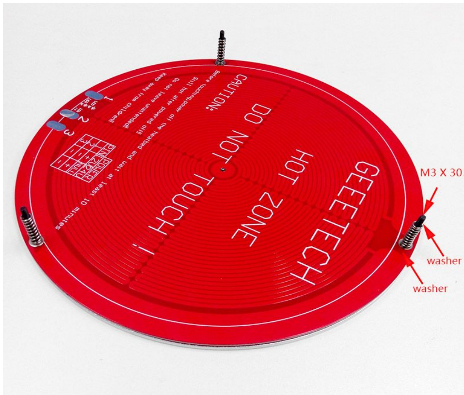
Step3. Lock the other end with a wing nut.
