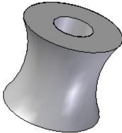
Figure 99: Drive wheel with a concave section acting as a constraint to keep the wrap in the centre of the wheel
