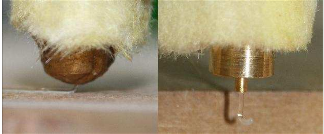
Figure 74: The original extruder nozzle was made from a bored dome nut (left) which exposed a lot of surface area to the build. The turned spigot nozzle (right) exposed less area to the build and attracted less debris.
