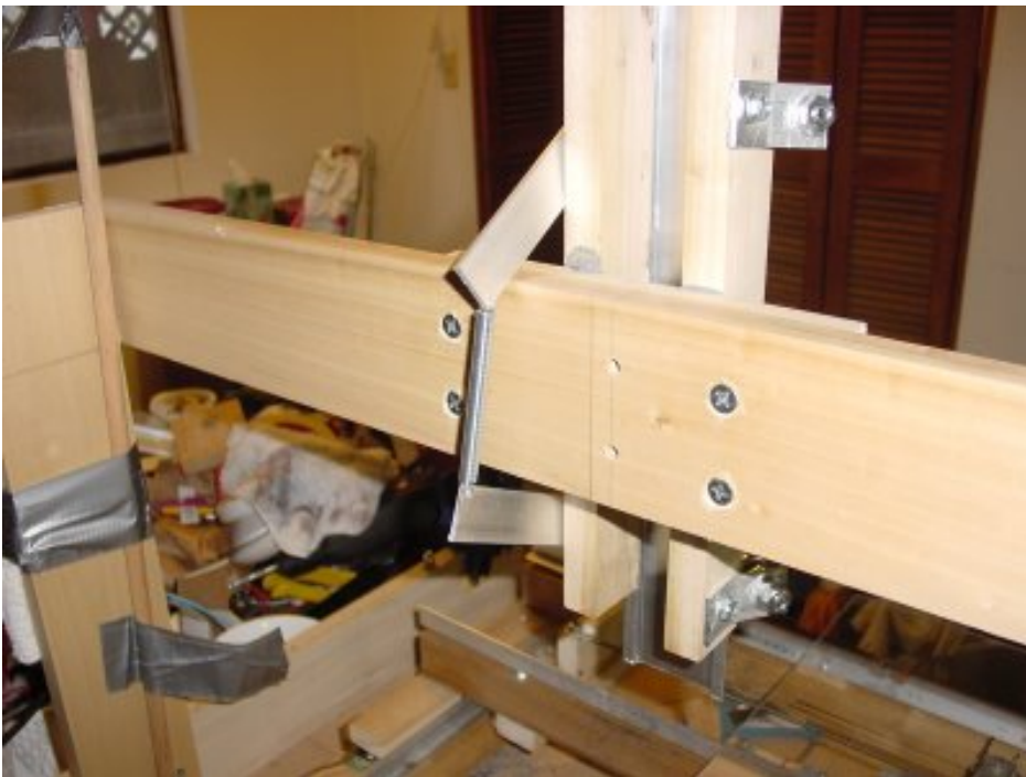
And here from the back side where you can see the tensioning spring for the bearings providing the normal compression.
