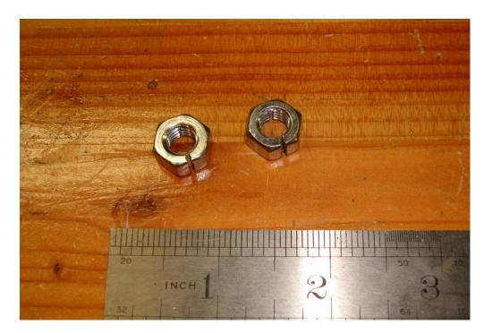
The result. This will be a jig to hold it in the 3 jaw lathe chuck.
