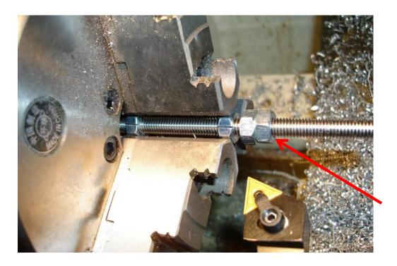
Put in the lathe and tighten jaws as shown. Note the cut clamps the rod firmly when the jaws are tightened. Lightly face the face shown, just a fraction of a millimeter by hand feeding across the face with the cross feed.
