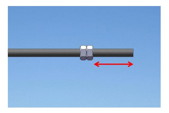
This step locks two M8 nuts together so the nearest face is 42mm from the end of the rod.
