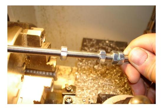
Now run the cut nuts on the rod, one near the locked nuts and the other the lathe jaw depth away.
