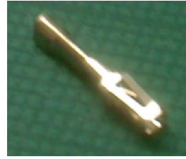
Figure 22 and Figure 23: A standard circuit board pin socket (with the connector section highlighted)
