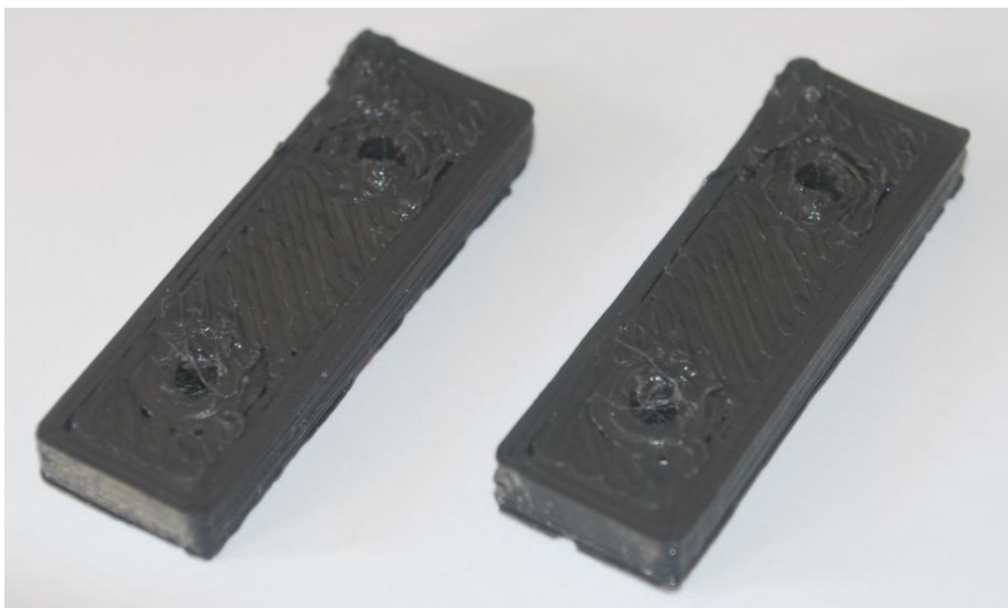
Figure 6-32 - MkI (left) and MkII (right) Active Nozzle prints with a 1:1 (black : white) ratio
