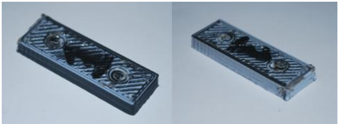
Figure 6-5 - First mixer nozzle print with very different appearance from opposite sides
