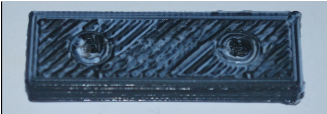
Figure 6-6 - Underside of first print, the extra shear caused between the nozzle and the print surface caused extra shear thus better mixing qualities
