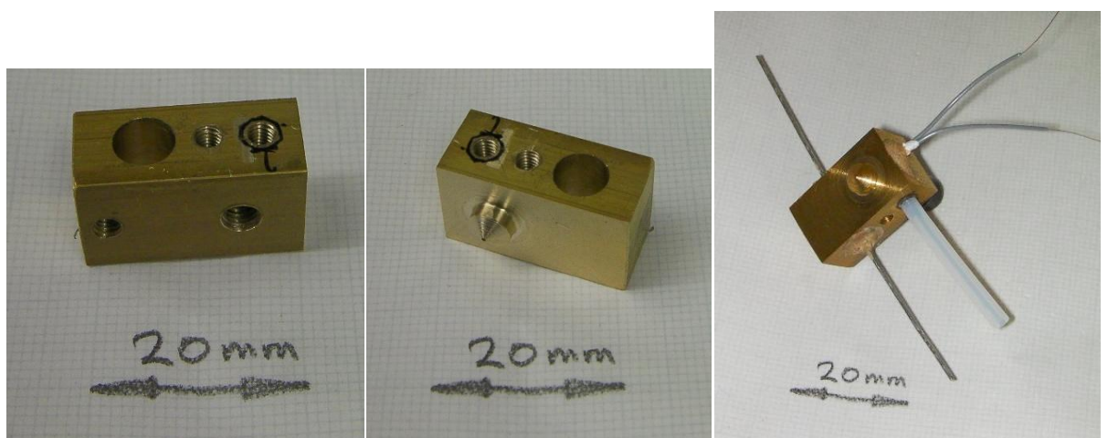
Figure 2-5 - The mixer extruder block for handling multiple materials [7].
