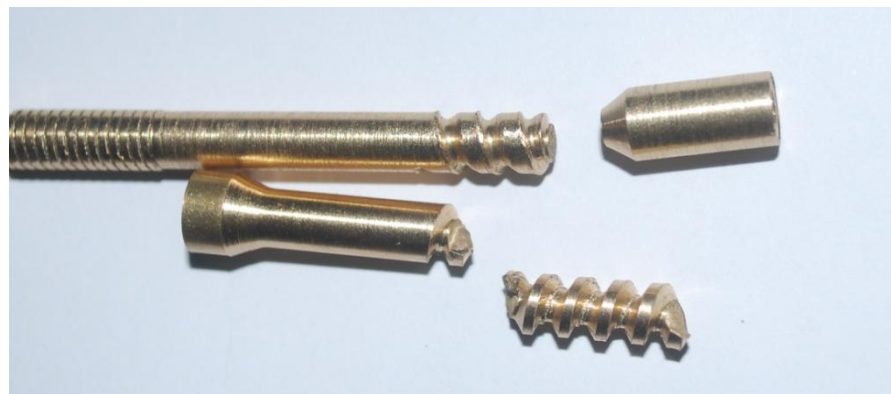
Figure 6-17 - Two examples of the brass failing during thread cutting due to lack of relief angle on the tool.
