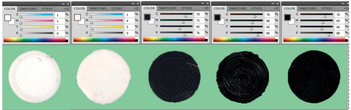
Figure 7-4 - Control White Print - C:1 M:1 Y:2 K:0 (far left), Mixer Nozzle White Print- C:1 M:4 Y:5 K:0 (left), Mixer Nozzle 1:1 White:Black Print- C:79 M:71 Y:60 K:76 (centre), Mixer Nozzle Black Print- C:76 M:68 Y:65 K:85 (right), Mixer Nozzle Black Print- C:76 M:69 Y:66 K:86 (far right)
