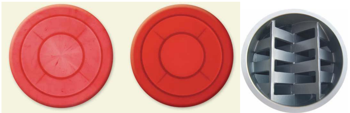
Figure 4-17 - Comparison between a standard nozzle (left), the Nickerson Static Mixing Nozzle (centre) using the same machine settings and a mixing element (right)
