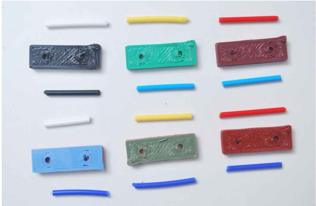
Figure 6-30 - Various colours mixes producing very identical quality prints with good mixing quality Appendix K
