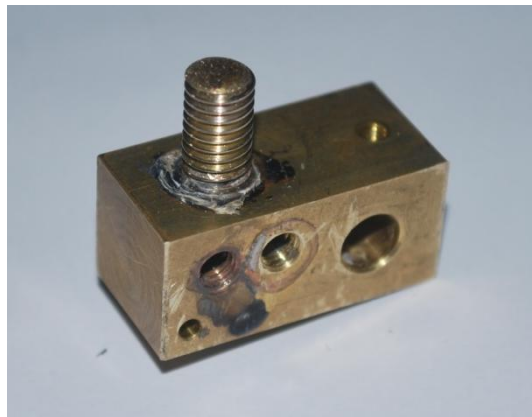
Figure 6-8 - MkII Brass mixing Nozzle with Mixing Chamber Brass Mixing Insert in Place
