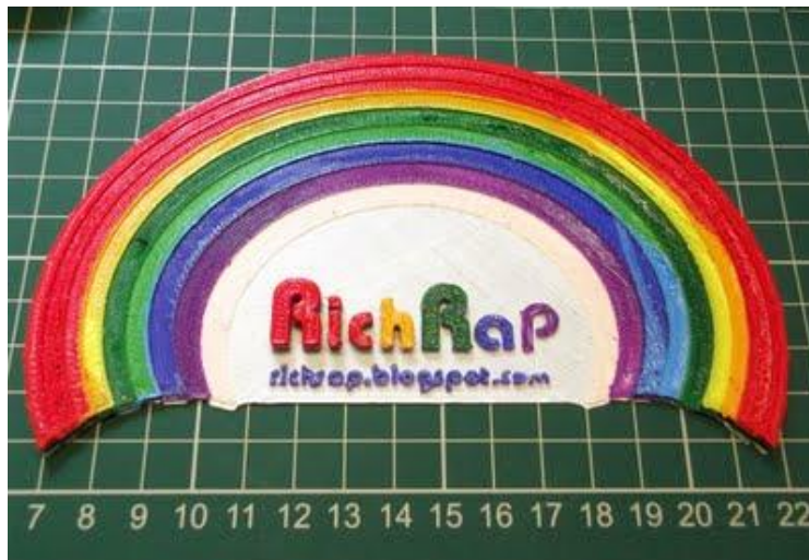
Figure 4-3 - Example of colour printing using filament joiner [9]
