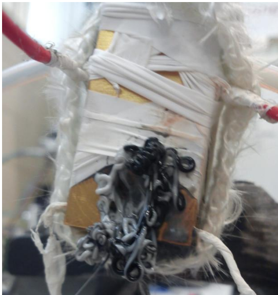
Figure 6-23 - Manual Feed results for the MkIV nozzle, white and black are clearly unmixed.
